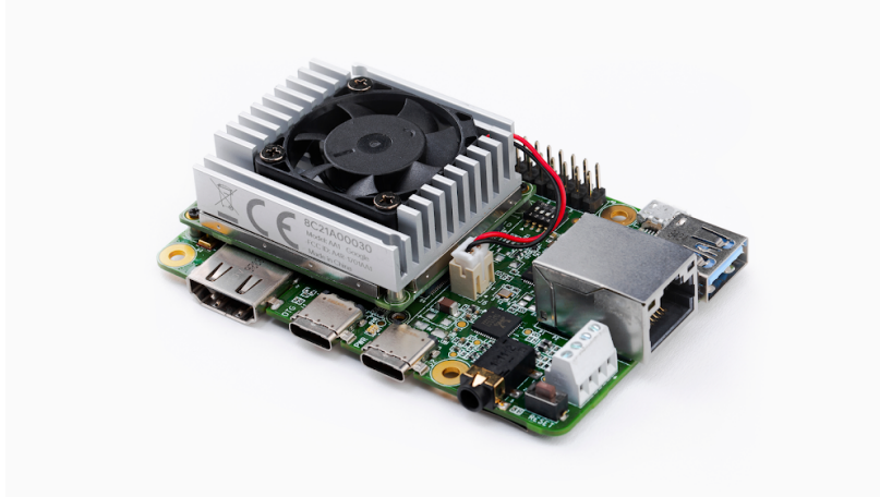
Figure 31: Edge TPU - Dev Board https://coral.ai/products/dev-board/
